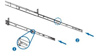
4 Remove the rails as the same way of installing. 依组装步骤拆卸导轨。
