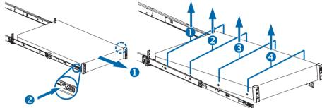
3 Press the side-release lock buttons on both rails and slide the rails into the rack.
