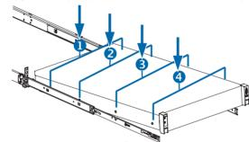
5 Press the side-release lock buttons on both rails and slide the system into the rack. 按压图中 ● 所示的导轨两侧卡扣,将服务器按照图中 ❷箭头所示的方向推入机柜。
