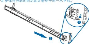
Repeat 1 and 2 steps to install the other side. And pull the inner rails out of the rack until they lock into place.
