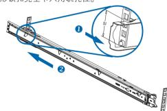
Pull up the latch release part on the front bracket. ❷Push the rail into the rack until the square pins are fully seated on the rack holes and the latch clicks into place. 将前固定件的释放件参照图中 ● 箭头拉开,再依图 ❷箭头将导轨推入,直到方形锁扣完全卡入角轨孔位。
