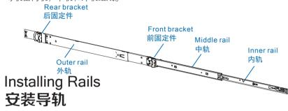
Position the rear bracket and align each pin with the rack holes. ● Pull the latch release button on the rear bracket. ● Push the rail into the rack until the square pins are fully seated on the rack holes and the latch clicks into place. 在机柜上确定好导轨后支架的安装位置,将导轨后支架上的方形锁扣和圆形按钮对准机柜角轨上的孔位,参照图中 ● 按压后托卡勾,再依图中 ● 箭头所示方向推导轨,直到方形锁扣完全卡入角轨孔位。
