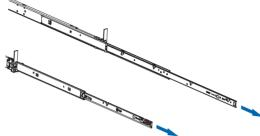
4 Align the rail standoffs on each side of the system and lower them into the slots on the rail. Put the system downward until all the rail standoffs are seated in the slots.
